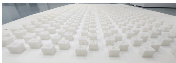
Where the magic happens. The ghost tunnel’s physical medium was an array of 15-mm-tall, partially hollow plastic elements. Credit: C. Xu et al. [1]
